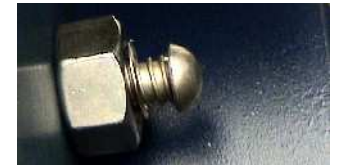
Flange lock pin located on back of blade guard.
