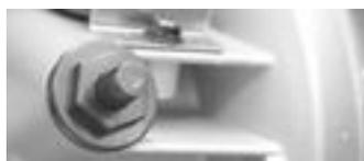
*Shaft lock pin located on front of motor.*
